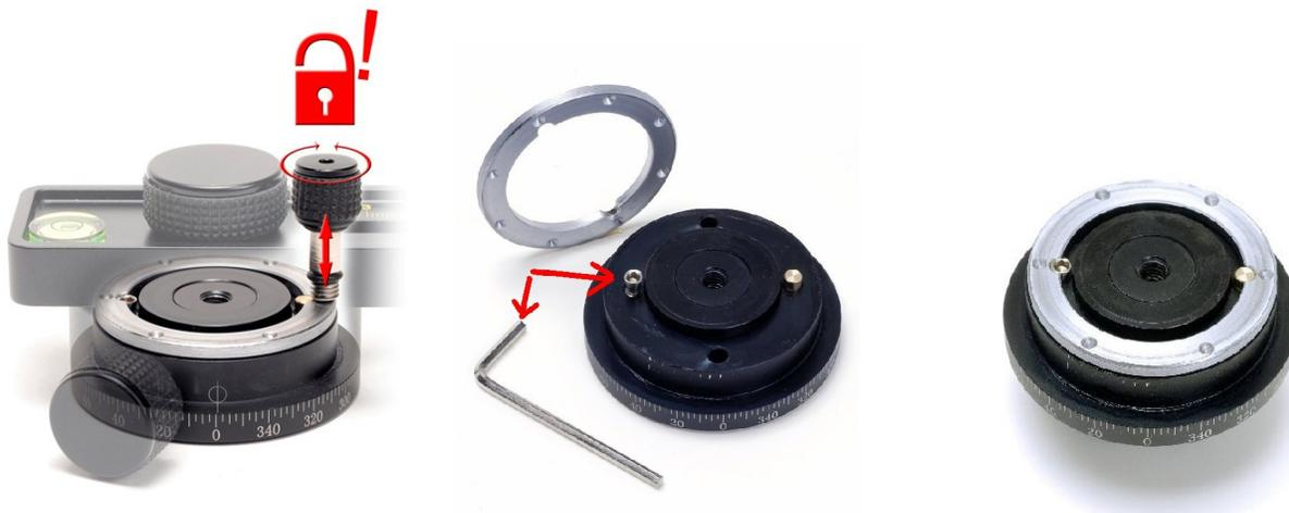
Using the enclosed hex key loosen the inner hex screw enough to release detent ring. Some units may have the hex key tool located inside the tension knob as shown above left. Place the detent ring with desired side face up. Tighten hex screw and reassemble.
