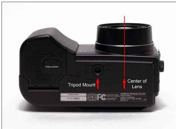
tripod mount is off center from the center portion of the lens you'll need to use the small camera bracket. If it is 20mm or less you can use the N3T20. If the offset is greater than 20mm and less than 30mm you can use the expanded N3T30 t-adapter. Using the t-adapter allows your camera to be positioned on the Nodal Ninja in such a way as to achieve proper rotation about a camera lens NPP. (NN3 used in sample images).
