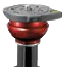
Center column with built-in 50mm half ball locked using the rotating grip located at the bottom of the center column. Tilt range: \pm 15^\circ .
