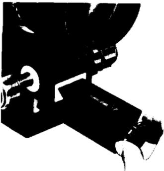
2. To remove the lens, depress the bayonet locking lever and turn the lens counter-clockwise until the two orange dots face each other.
